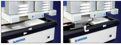
Pre-lidded plates descend individually (without the lid) from the original chimney, move to the dispenser for filling, and return to the original chimney to reunite with it's lid. The processed lidded plate is then moved to the chimney containing finished plates. (Pictured above with the WellMate and Plate Stacker.)
