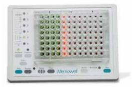
**384 Support**—Using MemoControl Software, a set of four wells in a 384 microplate can be illuminated. The image on the PC screen will then indicate which of the four wells is the desired target.
