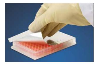
**Foil Seals**—For longer-term storage, light blocking, and the ability to pierce with pipet tips for sample access, foil seals are the ideal choice. The foil and adhesive are DMSO-resistant, apply easily, and are compatible down to -80°C.
